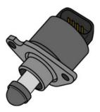
With a multimeter on the continuity setting, find the two pairs of terminals on the idle motor (the paired terminals are those which have continuity between them). Fit IDLE1 and IDLE2 on one pair, the IDLE3 and IDLE4 on the other pair. Within the pairings it does not matter which way round they go.
